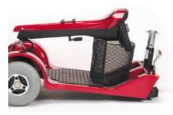
The tiller can be safely secured in position for transporting.
